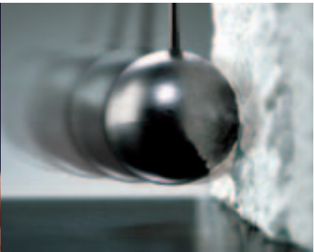
The pendulum test demonstrates StoTherm Classic's superior resistance to mechanical stress in comparison to mineral systems.
